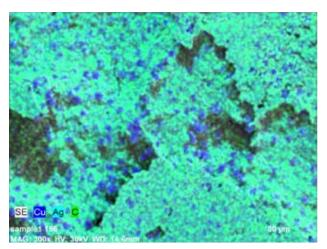
Figure 1. SEM image (left) of a Ag/Cu paste and the equivalent element map (right).
